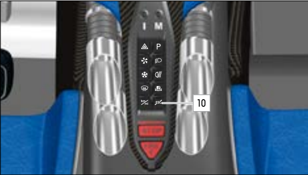
FIG.78 BUTTON FOR SWITCHING ON AND OFF THE ELECTRONIC STABILITY CONTROL (ESC) ON THE CENTRE CONSOLE
