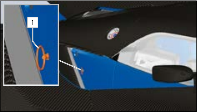
FIG.67 EXTERNAL FIRE EXTINGUISHER HANDLE ON THE OUTSIDE OF THE SIDE PANEL ON THE DRIVER AND PASSENGER SIDE
