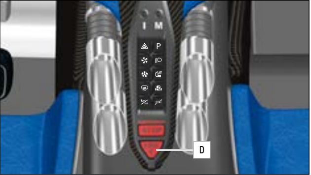
FIG.66 INTERNAL FIRE EXTINGUISHER BUTTON ON THE CENTRE CONSOLE
