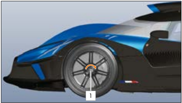
FIG.84 TIGHTENING DIRECTION ON THE DRIVER'S SIDE
