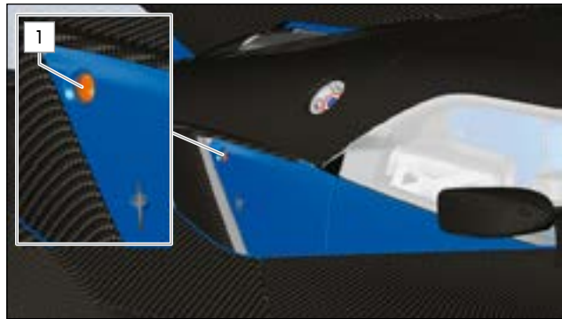
FIG.69 EXTERNAL STOP BUTTON ON THE OUTSIDE OF THE SIDE PANEL ON THE DRIVER AND PASSENGER SIDE
