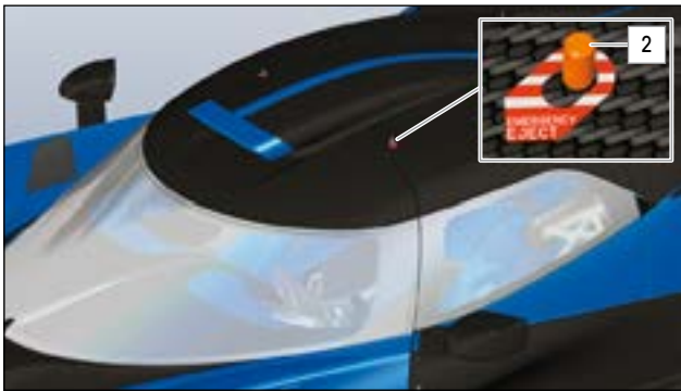
FIG.45 EMERGENCY RELEASE PIN ON THE DRIVER AND PASSENGER SIDE ON THE ROOF
